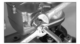
a) Install your fuel line into the BIG 97 S-jet inlet valve.
