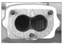
Modifying your intake manifold: Compared to a regular 97, the BIG 97 has bigger, flared throttle bores which form an oval plenum shape before they meet the intake. To make the most of this improved airflow capability, some intakes may need opening up around the bores and down into the webs between the two bores for each carburetor. You can use the supplied intake gasket as a template.
