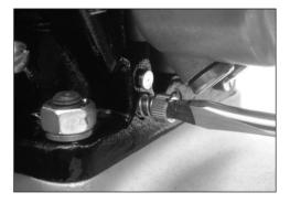
(counter-clockwise) to make the idle mixture richer (more fuel). Turn each idle screw in slowly (1/4 turn at a time) until the engine begins to lag or run irregularly. Then turn the same screw out slowly until the engine begins to roll or gallop, then back in slightly to provide the smoothest idle. Repeat this same procedure to adjust the other screws. Be prepared to go around all of the screws again if required.
