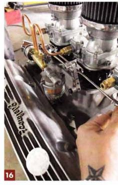
Even though an electric fuel pump will be used, which would normally give the option of running the fuel lines toward the front or the back of the engine, with oil filler tube combined with the tighter confines dictated by the progressive linkage, going backward was really our only option.
