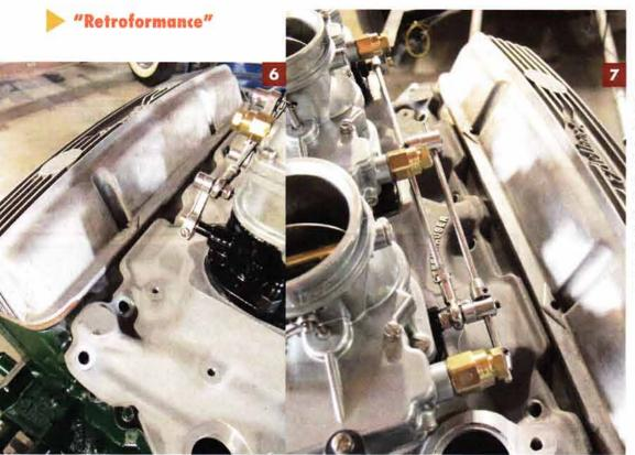
... make sure there'll be no interference between either component. If you look closely, you can see that had it not been for someone previously notching the inner lips of the valve covers, the thicker intake runner flanges on the Offy manifold wouldn't have cleared.
