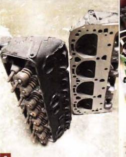
Gone are the high-swirl center-bolt cylinder heads to make room for a set of pre-'87 standard cast-iron heads. Note that neither the base engine nor the new (old) heads are performance-oriented to begin with — if we were looking to achieve big numbers, we wouldn't have chosen either in the first place. This will be good, reliable, and as efficient an engine as can be.
