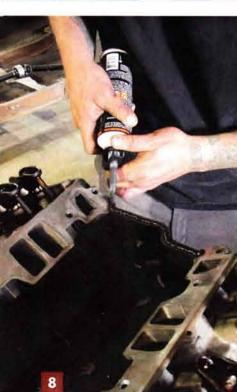
With the clearances all cleared, the sealing could finally begin. Rather than using cork or rubber front and rear seals, a nice big bead of silicone was laid on the block from head to head. Normally, this prevents leaks better, as the seals sometimes have a tendency to get pushed out when the manifold is tightened down.
