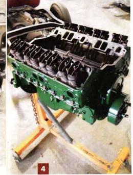
Heads installed and valvetrain initially dialed in, it's time to pre-fit the intake system. One thing about this particular engine that we learned (were told) was that despite having an external fuel pump provision, there is no internal provision to run a mechanical pump — which won't pose a problem since an electric fuel pump will be used.
