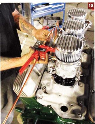
18 And unlike the aforementioned Caddy setup, the addition of a third carburetor posed a small challenge with routing the rear fuel line in a similar fashion as the front and center lines. More than likely, the overall configuration will be changed once the engine's in the vehicle and we have a better idea of how the surroundings (firewall mainly) will apply.
