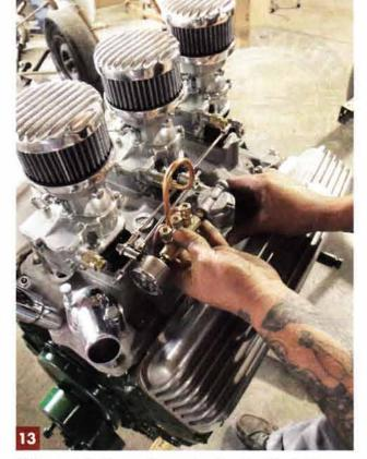
First we needed to figure out the overall configuration of the fuel lines. Things taken into consideration: linkage clearance, manifold/valve cover clearance, and what direction the fuel supply would route.
