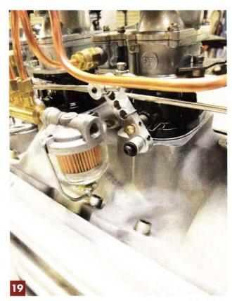
Throughout the entire fuel line process, one thing we constantly checked was that there was absolutely no interference with the linkage — period. Ample room was left so that the throttle arms would have full range of travel.
