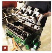
And as with the previous process, there's more than one way to skin a cat when it comes to intake manifold gaskets. In our case, the gaskets were first attached to the head with Gasgacinch, then a dab of silicone at each corner between the block and head, before the intake was dropped in place (no dressing on top side of gasket).
