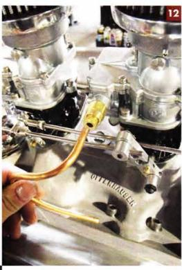
Now that the manifold's in place with the Strombergs all set up and ready to go, all that's left now is to install the fuel lines, brass fuel log, glass bowl filter, and pressure gauge. SO-MO provides compression fittings with their fuel supply systems, so no tube flaring is necessary.
