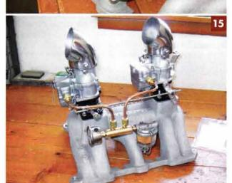
Here's an example of how SO-MO did the fuel lines on a Caddy 2x2 Widow Maker, Note that the lines feeding the carburetors run up vertically from the log before turning into the fuel inlets rather than being a straight shot over as with other types of supply setups.
